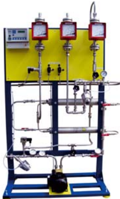
Figure 2. Filtration unit with 2 SR-1 elements. Capacity is 25 L/h. Filtration performed at 35 °C.
